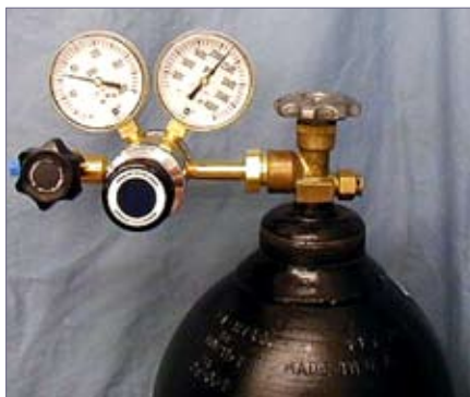
Figure 1. Typical installation of a regulator on a cylinder.
