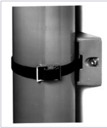
Figure 2. Prior to attaching the regulator, make sure that the cylinder is properly secured to prevent it from falling.
