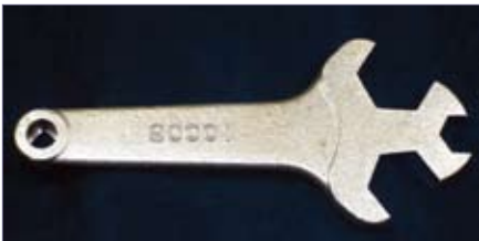
Figure 3. Proper regulator tightening wrench.
