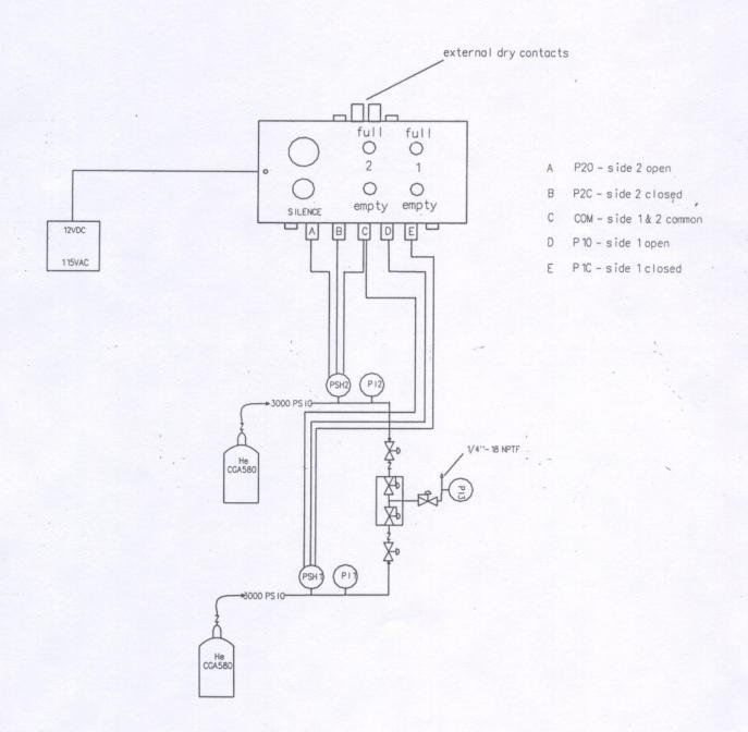
PSH1, PSH2 PRESSURE SWITCH SET POINT • 300 +/- 25 PS IG PI1,PI2 PRESSURE GAUGE 3000 PSIG PI3, PRESSURE GAUGE 200 PSIG
