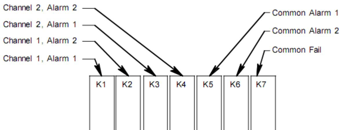
**Figure 3. Beacon 200 Channel Relay Allocation**
