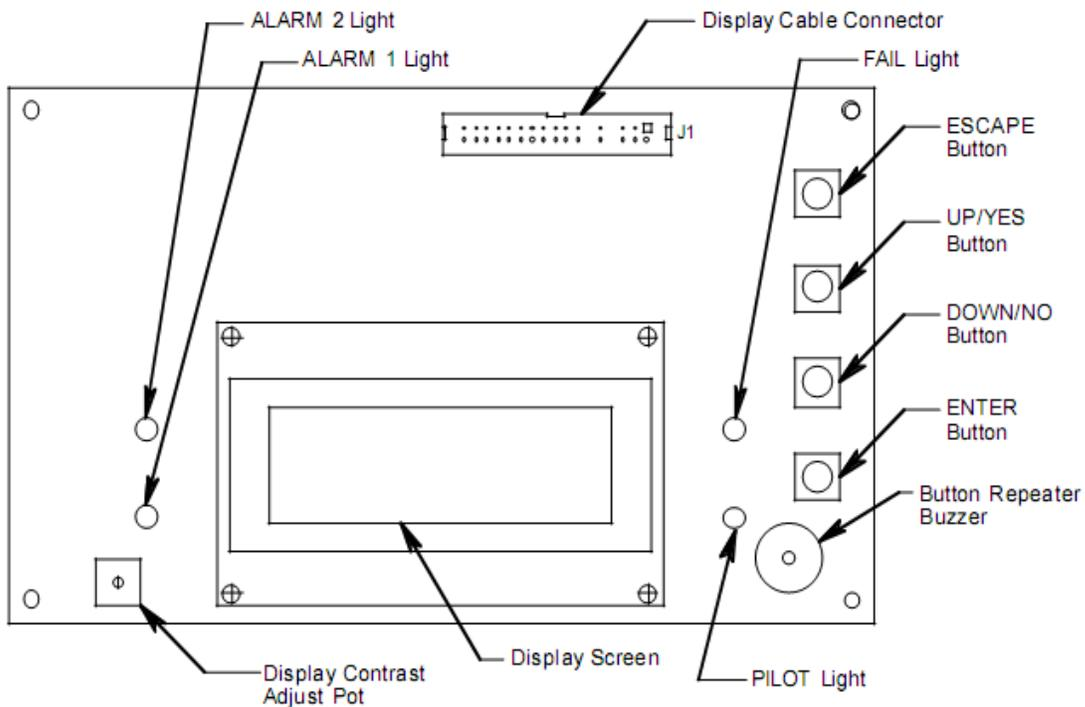
**Figure 2. Display Board Component Location**
