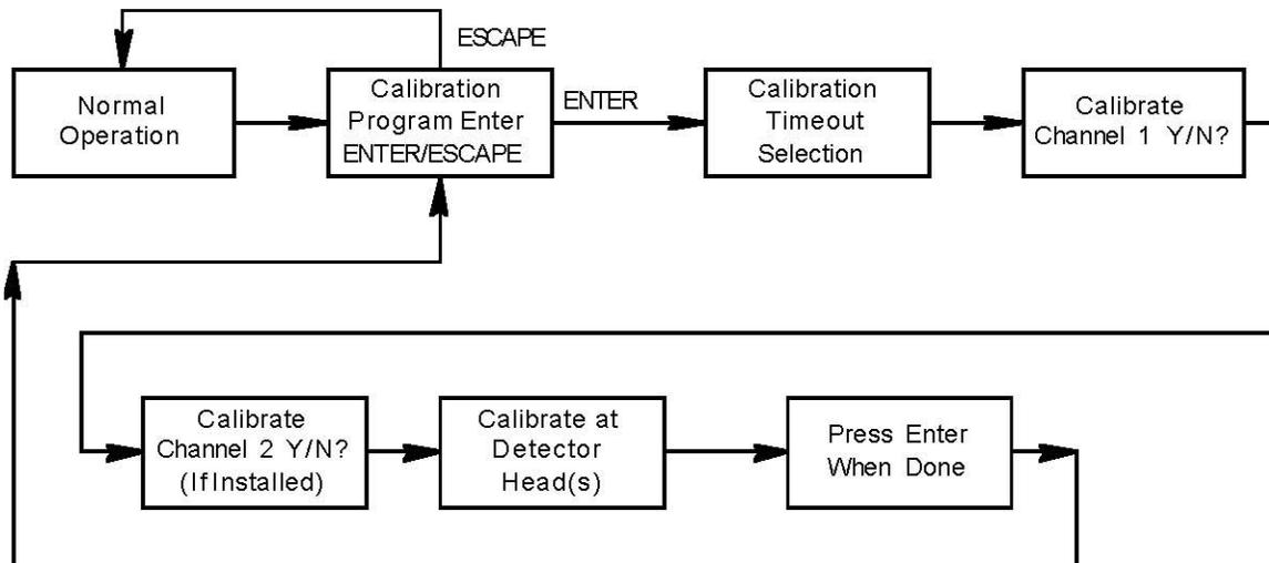
Figure 12. 4 - 20 mA Transmitter Detector Head(s) Only
