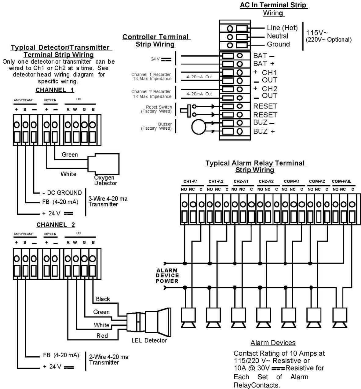
**Figure 5. Beacon 200 Gas Monitor General External Wiring Diagram**
